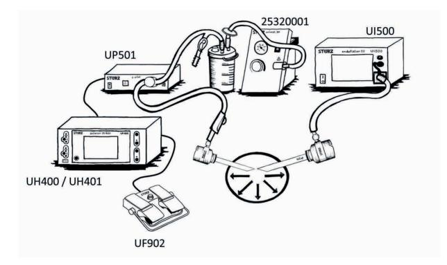
**25**320001 UNIMAT® 30, Suction Pump Set, power supply 230 VAC, 50/60 Hz including: **Bacterial Filter** Secretion Bottle **Bottle Cap** Connecting Tube, short **Patient Tube Overflow Case** Mains Cord, length 300 cm UI 500 S1 ENDOFLATOR® 50 SCB, with integrated SCB module, power supply 100-240 VAC, 50/60 Hz including: SCB Connecting Cable, length 100 cm **Universal Wrench** Heated Insufflation Tubing Set, with gas filter, sterile, for single use, package of 3 HICAP® Trocar, size 11 mm
