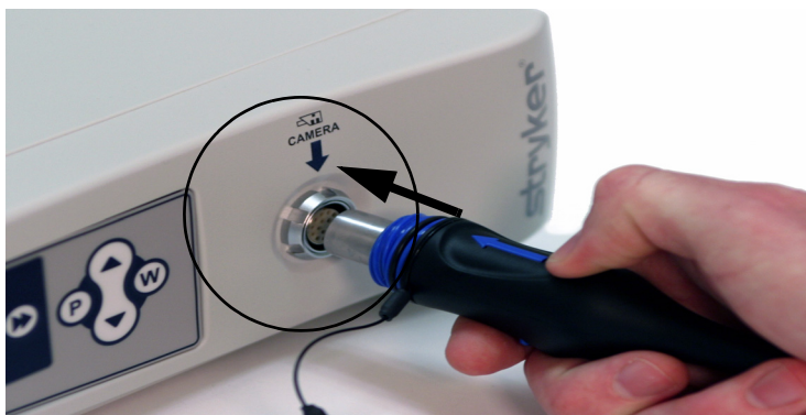
Figure 4: Connecting the camera head to the console
